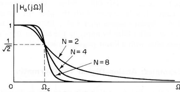
Fig 1: analog Butterworth filter (low-pass)
